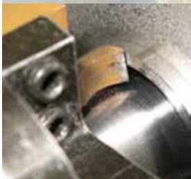
Exact squaring and beveling through the use of up to four extremely inexpensive tool bits (available optionally).
