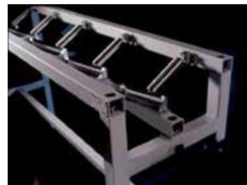
Pipe feeder for accurately feeding long and heavy pipes into GF and RA machines (page 22)
