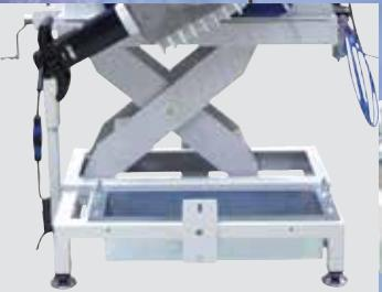
Including a height-adjustable and robust lifting bench with a container for swarf collection
