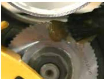
Our high-performance lubricants for cutting and beveling to increase the tool life of saw blades (page 20)
