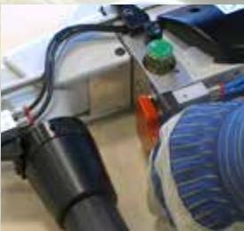
Automatic starting of the working process (pipe clamping and machining) with only one tip switch.
