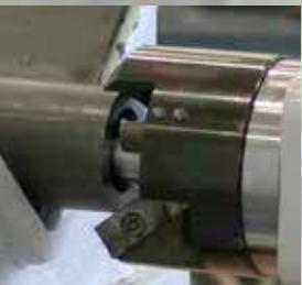
Standard-compliant, precise and reproducible weld seam preparation.
