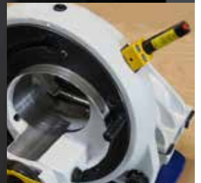
Integrated line laser to mark the cut off point
