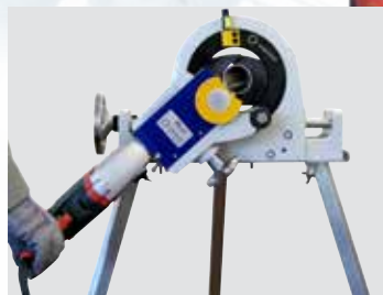
Cutting thin-walled stainless-steel tubes and elbows
