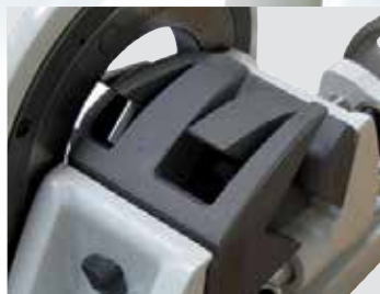
Deformation-free clamping of thin-walled tubes
