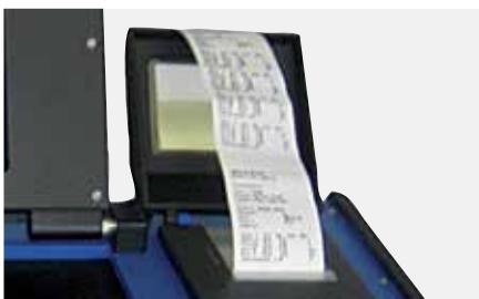
*Integrated job printer allows actual values to be printed out*
