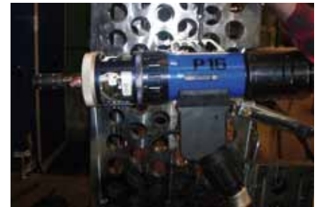
Internal bore welding (I.B.W.)
