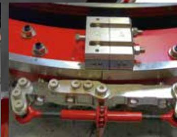
Designed to split into quadrants without sacrificing rigidity, swing bolts and a ratcheting hinge mechanism speeds assembly and mounting.
