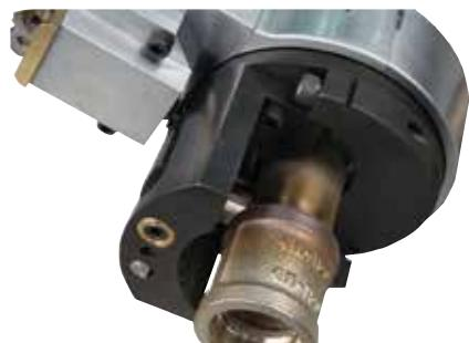
Axial slide for socket weld removal
