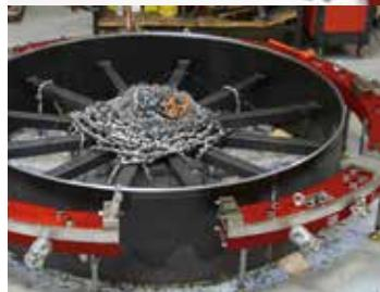
Four standard LDSF sizes cover a range of 60" to 120" (DN1500-3000) OD with a 15" (381 mm) capacity between sizes.
