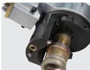
Axial slide for socket weld removal.
