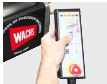
Control machine power and rotating speed from distance away with the hand pendant.
