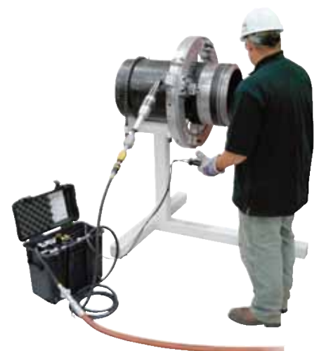
ACM controlling Low Clearance Split Frame
