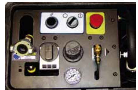
Ergonomic fingertip control for all air functions with safety stop button.
